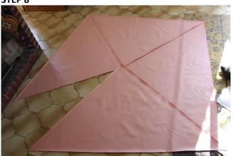
Cut up the 4 parts of the canopy in the textile Sew the 4 parts together Insert eyelets at each corner (4) of the canopy
